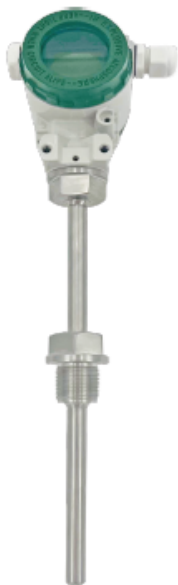
Thermocouple temperature transmitter SHT-WZP Graduated mark: PT100 / K / S Output: 0-10VDC, 4 ~ 20mA, 4 ~ 20mA+Hart Measuring range: 0 ~ 1300°C
